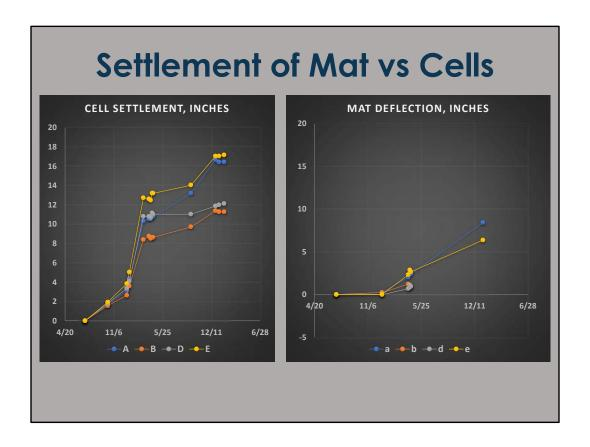
The two south corners of the mat had deflected upwards about 5.2 and 6.8 inches. This deflection must have involved a structural failure of the foundation.
