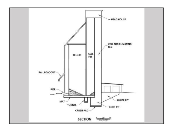
Trucks would drive through a covered dump house and dump their grain into sloping pits that would feed by gravity into the base of the elevating leg. The base of the leg would be enclosed in a "boot pit" extending 16 feet below the main foundation slab.
