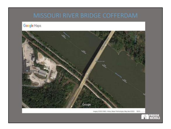
The topography and geology varied greatly along the length of the proposed bridge. The Nebraska (west) side was a high bluff with limestone bedrock just a few feet below the ground surface. Shale and limestone were found about 16 feet below the water surface at the west bank. The lowa side was a floodplain with a few feet of clay and silt at the surface, underlain by up to100 feet of sand over bedrock.
