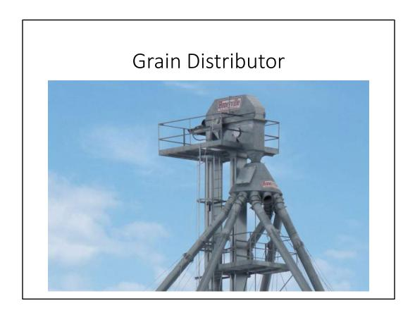
At the top of the leg, the grain falls into the distributor, which directs the grain into one of several chutes leading to storage cells, other storage structures, and truck and railcar loadouts. The leg can move grain rapidly to keep up with the rush of trucks bringing the harvest from the farm fields.
