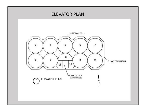
The cells would be interlocked, slip-formed concrete founded on a rigid reinforced concrete mat foundation about 2.5 feet thick bearing 4 feet below the ground surface.
