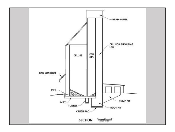
The tunnel and boot pit slabs were cast on bales of straw to prevent the slabs from being overloaded as the soil compressed. The mat was cast on a 12-inch-thick layer of sand to encourage vertical drainage during consolidation.
