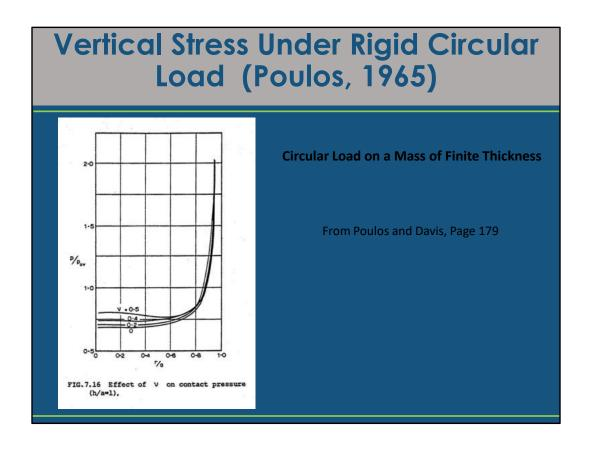
A rigid foundation cannot bend to conform to the dish-shaped settlement profile that a uniform load creates. As the soil compresses, the rigid body transfers load to the edges, and the applied soil pressure becomes nonuniform. Some textbooks show examples of the pressure distribution under a rigid foundation. This one is by Poulos.
