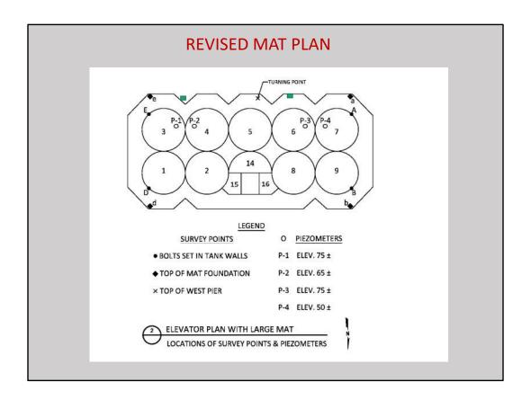
The tunnel, boot pit, and mat were constructed. Crosses were chiseled in the top of the mat near each corner, and the elevations were determined by differential levelling from a frost-free benchmark.
