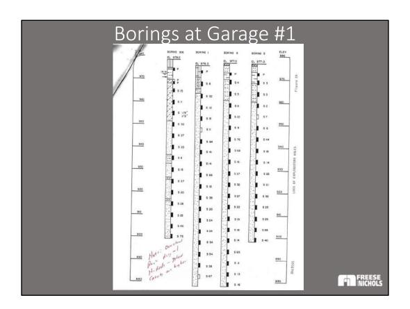
The airport is located in the floodplain of the Missouri River. Typical subsurface conditions consist of surface layers of weak silty and clayey soils underlain by loose to very dense fine to medium sand. At the project site, the sands extend more than 100 feet to bedrock.
