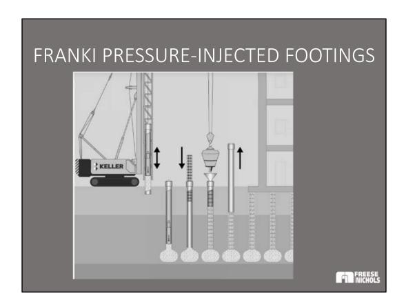
Franki PIFs are installed by driving a heavy steel casing using a 5-to- 10-ton cylindrical drop hammer.
