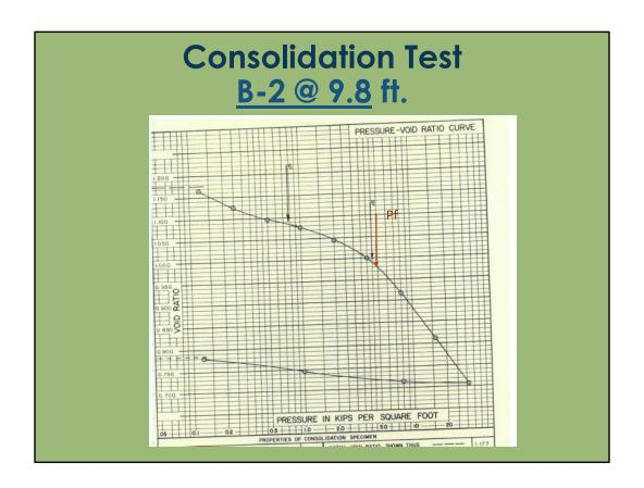
Consolidation tests showed the loess to be moderately overconsolidated, with preconsolidation pressures of about 4 to 6 kips per square foot.
