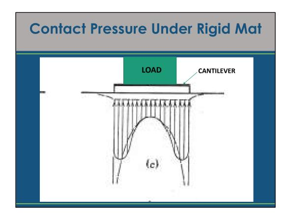
According to elastic theory, the pressure approaches infinity at the edge. This will not occur on a real soil because the soil will shear and move out from under the edge.
