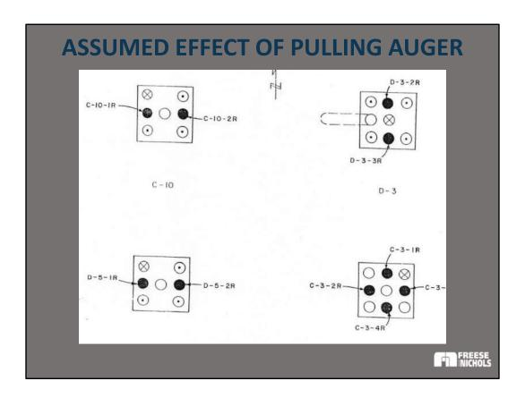
Previously placed piles adjacent to a re-augered pile were assumed to have negligible capacity. Piles added after the re-augered pile were assumed to have full design capacity. Steel piles were added to make up the lost capacity and provide balanced support. It was assumed that the heavy steel piles bearing on rock could provide more than 120 tons support if needed.
