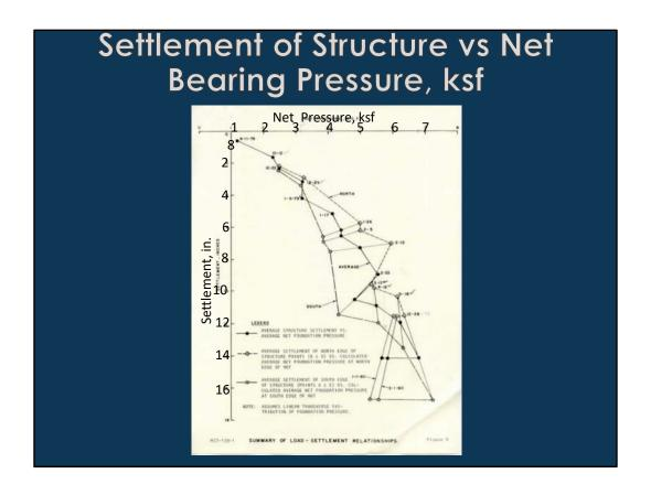
Settlement, tilting, and pore pressure changes were closely monitored. Initial filling of the structure with grain took two harvest seasons. The elevator had a persistent tendency to tilt southward. More grain was placed in the north tanks to counteract the tilt, but when all the cells were full, the average settlement was 14 inches, and the tilt was 17 inches at the top of the cells.
