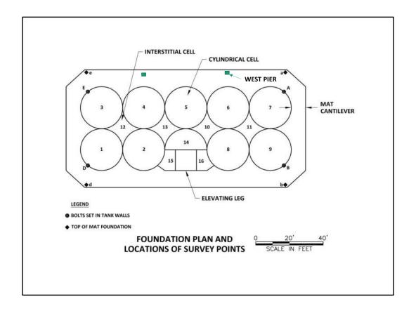
A pier supporting a railcar loading chute was used as a turning point as the surveys were looped around the structure. It was noticed that the turning point was not settling as much as the two anchor bolts on the southeast and southwest corners of the elevator, suggesting that the cantilever of the mat foundation might be deflecting upwards. Steel rods were driven to the top of the mat and surveyed as time went on.
