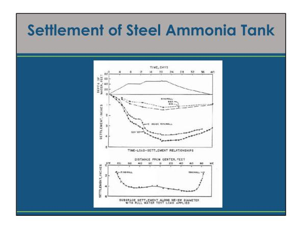
An example of a uniformly loaded area is a thin-bottomed steel tank. This chart shows the measured settlement of a 170-foot diameter tank filled with 50 feet of water.
