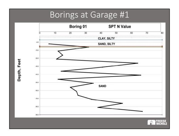
As usual, SPT tests showed that the sand formations deposited by the river are highly variable in relative density. Much of the sand has SPT N values in the medium dense range, between 10 and 30 blows per foot. Other layers are dense or very dense, with a few values exceeding 70 blows per foot.
