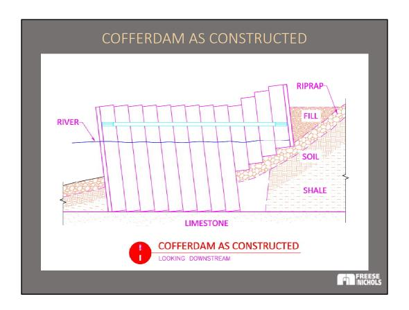
The cofferdam had wracked and tilted towards the river. The excavation was short of its design width on the landward side. Some sheet piles had refused on the riprap.
