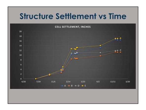
This chart shows the settlement of the four corners versus time. The south side settled about 4 inches more than the north side.
