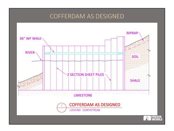
The cofferdam would be about 40 by 60 feet in plan. It was to be built using Z-section steel sheet piles driven through the shale to the limestone. It would be braced using 36-inch wide-flange beams serving as wales and struts.
