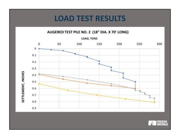
Test piles confirmed that the desired 120-Ton capacity could be obtained.
