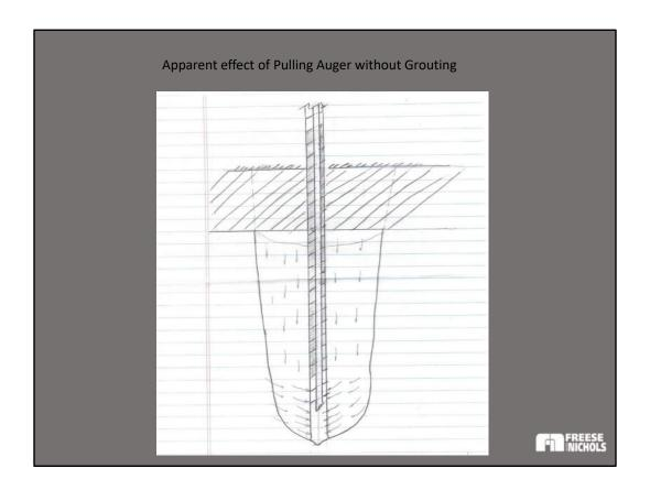
We concluded that withdrawing the auger without grouting loosened the sand to a distance of more than 5 feet away.
