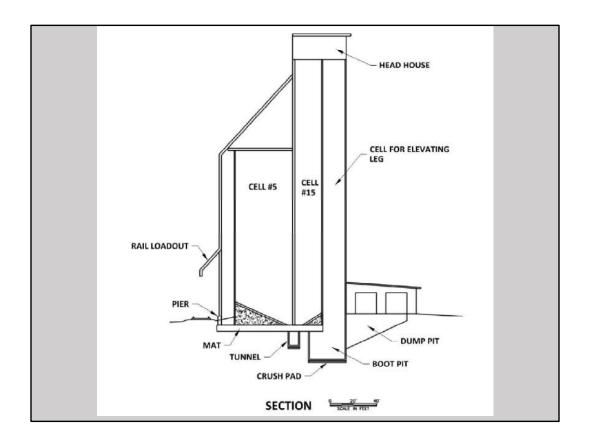
The cells would be unloaded by gravity flow onto a horizontal belt conveyor in a 7-foot-square concrete tunnel running under the center of the mat.
