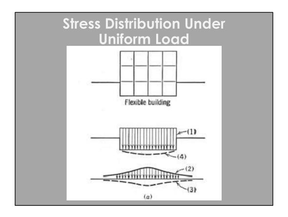
Elastic analysis shows us that an area loaded with a uniform pressure tends to cause higher pressure at the center and lower pressure at the edges on a plane at substantial depth. The foundation will tend to become bowl-shaped.
