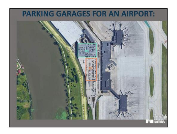
About 1984, Eppley International Airport wanted to build their first multi-story parking garage. It would have 6 parking levels with allowance for 2 future additional levels. Construction would use prestressed concrete columns, beams, and double-tee floor panels. Design column loads would range from about 900 to 1800 kips. Ten years later, a second garage of similar height was constructed immediately south of the first garage./
